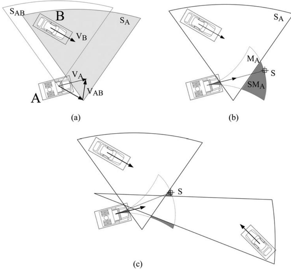
**Figure 2** An example of the avoidance maneuver algorithm as implemented in the SAFEPED according to Fiorini and Shiller (1998), where more details can be found.
