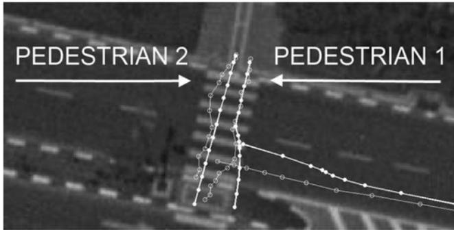
**Figure 5** Distant (a) and close (b) view of the trajectories of pedestrians and the car extracted from the video clip (gray) and simulated by the SAFEPED (white).
