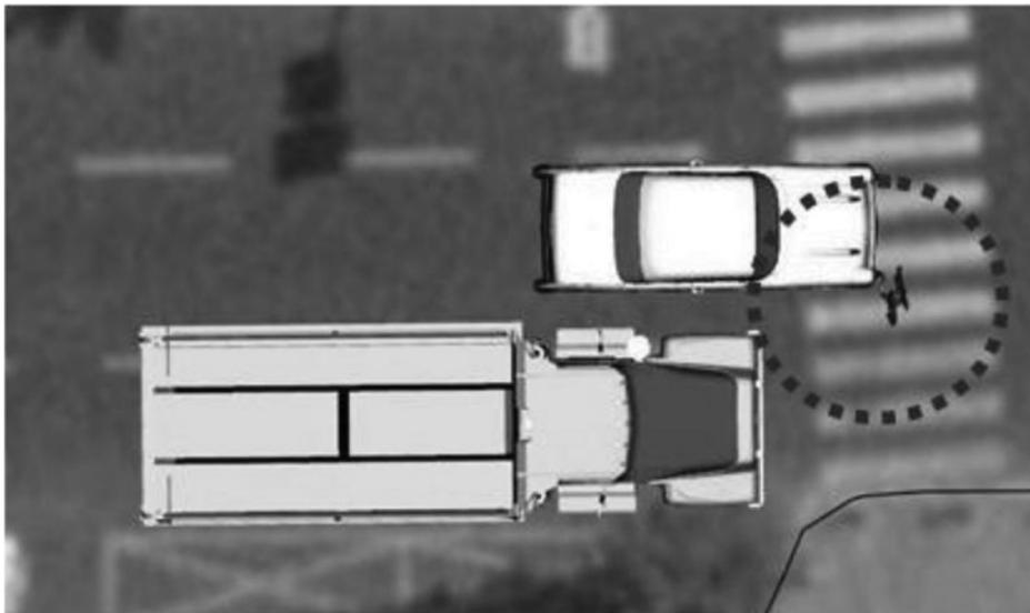
**Figure 12** Car's right fender hits pedestrian when truck is parked 0.75 m from the crosswalk.
