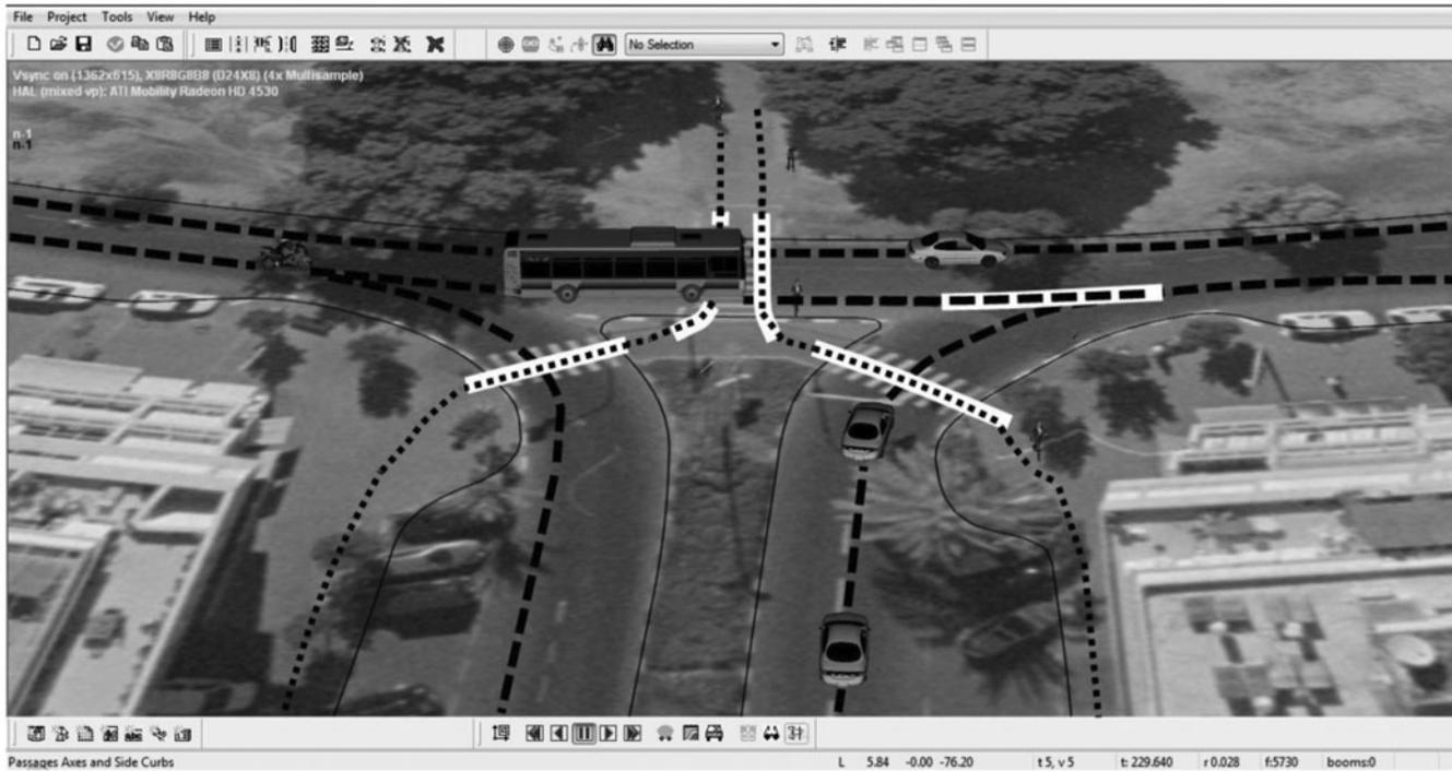
**Figure 1** SAFEPED model scene showing agents' trajectories. Dashed and dotted lines represent vehicle and pedestrian trajectories, respectively. Highlighted intervals represent the areas of possible interactions between vehicles and pedestrians and the priorities.
