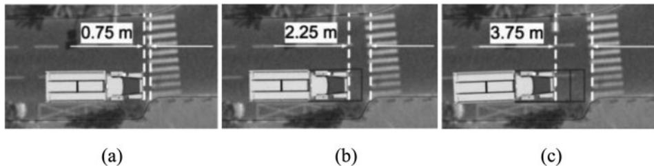
**Figure 11** Three experimental situations: The truck stops at a distance of 0.75 m (a), 2.25 m (b), and 3.75 m (c) from the crosswalk border.
