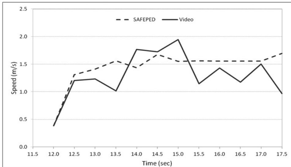
Figure 8 The speed of Pedestrian 2 in reality and in the SAFEPED simulation.
