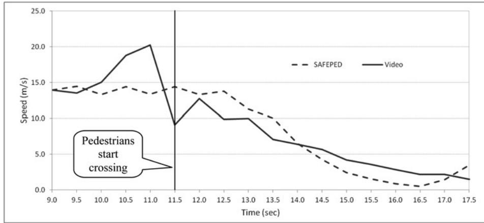
Figure 6 The speed of the car in reality and in the SAFEPED simulation.
