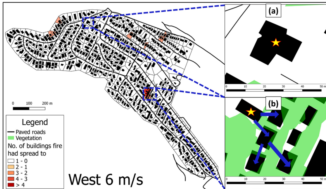
Fig. 10. (Left) the average number of buildings a non-extinguished fire had spread to within 1 h for 6 m/s north wind, by building of origin; (a) fire spread around low-risk location; (b) fire spread in 1 h around the most risky location.
